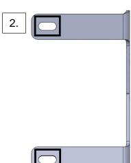
3. With a 10mm socket and T40 Torx, install the passenger side light bar bracket to the roof using the 2 removed T40 bolts and the included nyloc nuts and washers. Leave the bolts loose to allow for adjustment. Repeat steps 1-3 for the driver side of the vehicle.
